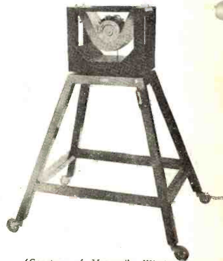
(Courtesy of Marconi's Wireless Telegraph Co., Ltd.) Fig. 6. The microphone and its stand in the broadcast studio of station 2LO, London. This is supported on a soft rubber cushion which absorbs all vibration.
