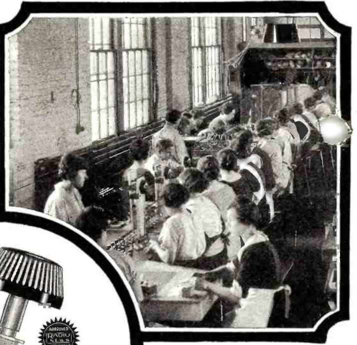
View of one production line, showing operators assembling Bradleystats and packing them in cartons for shipment. All parts are fabricated in other departments. The electric furnaces are in a separate building.
