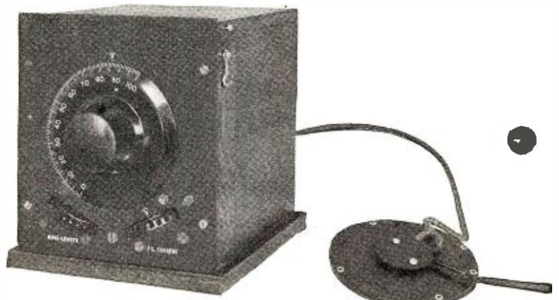
Fig. 2. A front view of the Clarifier and its output coupling coil.
